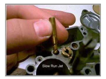
This is the slow running jet, check it for grime, use carb cleaner and compressed air to clean it out. DO NOT PUT METAL OBJECTS IN THE JET TO CLEAN IT! Refit the jet and tighten until SNUG, no tighter.
