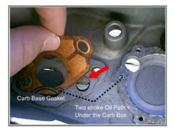
We're finished the carb rebuild. You can continue to this step if your engine has seized from lack of oil, if your Oil Device is working, DON'T MESS WITH IT and put everything back together. First, remove and plug your oil line with a bolt. To remove the Oil Pump body, undo the three screws and loosen the plumbing.
