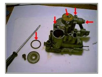
Once you loosen the nuts, Pull the Carb body STRAIGHT UP and out of the box. You will now be looking at your CRANKSHAFT! Put a little lint free shop towel over the intake port opening (towel omitted for clarity) dropping screws down into the crankshaft would be BAD! The gasket over the opening is the carb to base gasket.
