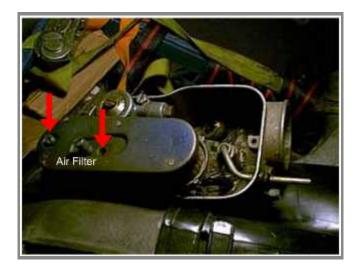
Run your bike with the gas off until the engine dies. Start by removing the screws arrowed, this will remove the Carb Box cover to reveal the meaty, juicy insides. When you re-tighten these screws, do it evenly to avoid warping. When you remove the cover, be gentle, there is a rubber seal under the lid. Inspect the seal for cracks; if it is missing or cracked buy a new one.
